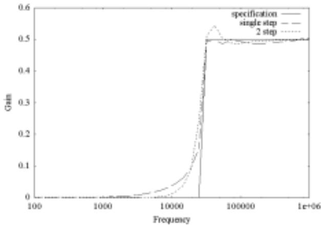
Figure 7: Specification and Acquired Response of High-pass Filter
