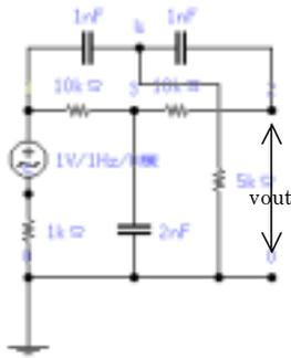
Figure 3: Band Elimination Circuit Design
