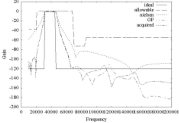
Figure 4: Acquired Asymmetric Bandpass Filter Response
