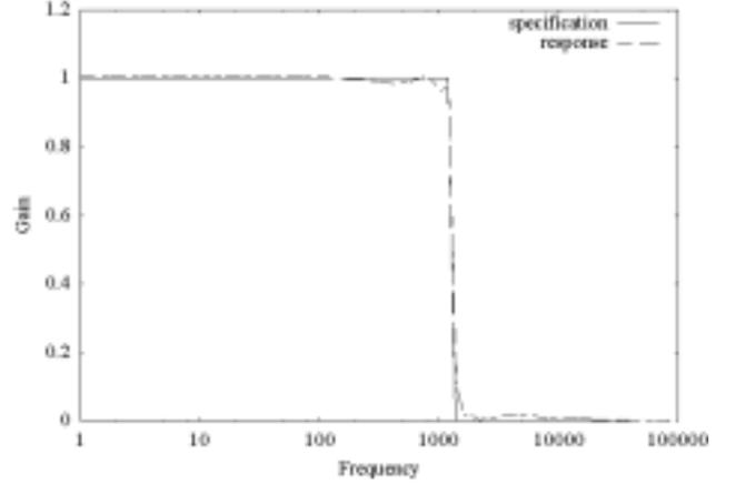
Figure 5: Specification and Acquired Response of Ideal Lowpass Filter
