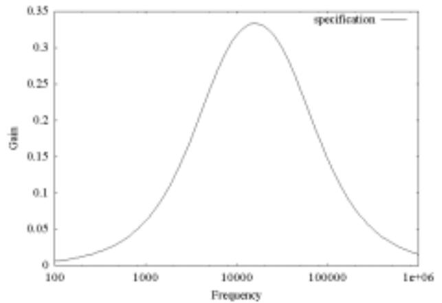
Fig. 9: Objective Bandpass Filter Response
