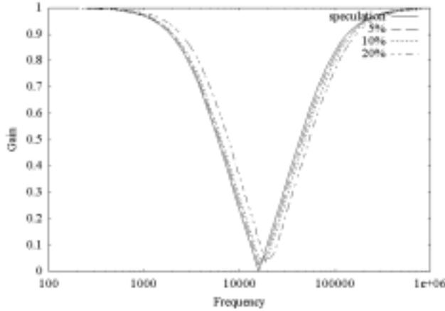
Figure 2: Ideal and Actual Response of the Band Elimination Filter
